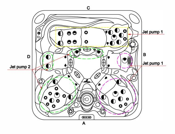
Notes:Due to manufacturing tolerances, there could be some minor differences between the actual spa and the drawing above. If also planning is critical to such tolerances, be sure to measure your actual spa. All specifi
