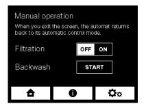
Manual control allows to: switch filtration on/off independently to preset filtering
