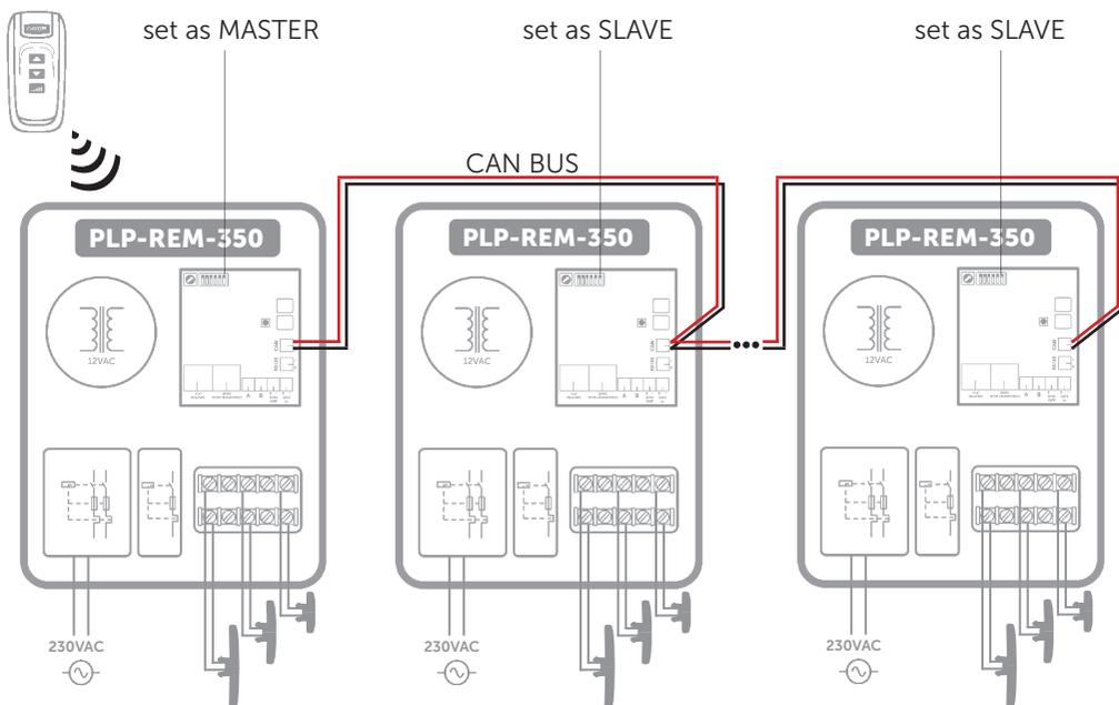
\* We recommend using a shielded twisted pair cable (min. 0,5mm<sup>2</sup> - up to 200m) to connect multiple PLP-REM-350's using the CAN bus.
