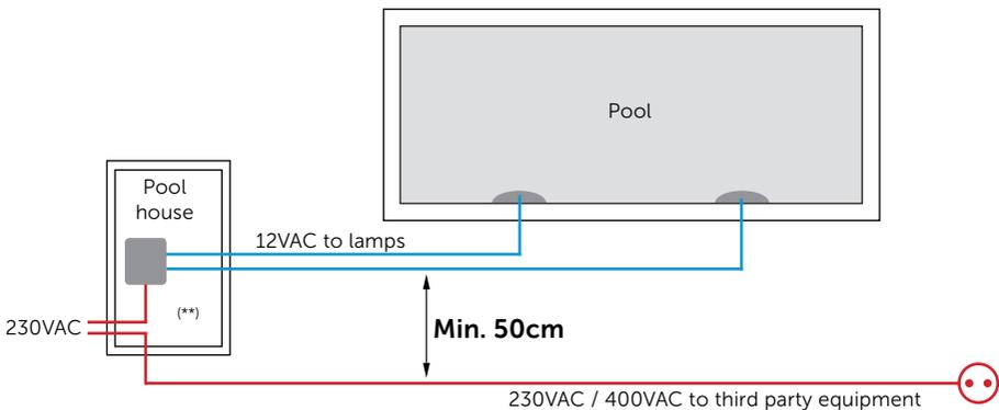
**(\*\*) Do not mix 12VAC and 230VAC / 400VAC power line cables into the same cable trays**
