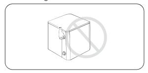
1.4.3. Don't put obstacles before the air inlet and outlet of the heat pump.
