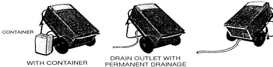
8. (i) Permanent Drainage: Normally a typical garden hose is utilised (12mm bore) . Bear in mind, drainage relies on GRAVITY FLOW so ensure a constant 'FALL' away from unit. In very cold weather, the water in the hose may freeze and 'back-up' through the unit to cause overflow.
