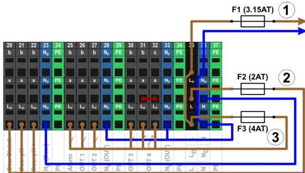
The supply for the PoolManager® unit as well as for the alarm relay and the add-on functions share a mutual power input (L/N). Phase L for PoolManager® is run from the input over via fuse F1. Phase L<sub>F</sub> for the alarm relay and the add-on functions is run from the input via fuse F3. Neutral conductors N and N<sub>F</sub> are connected to each other internally.
