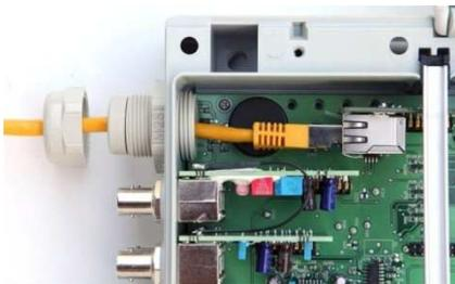
8. Press the rubber seal into the cable fitting.
