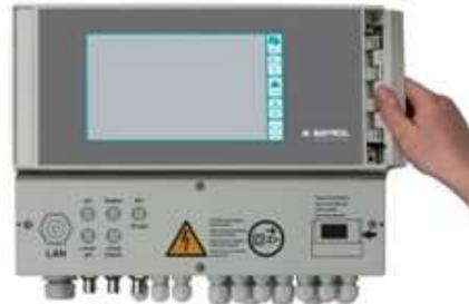
2. Remove the cover plate and unhook the hinge on the bottom.
