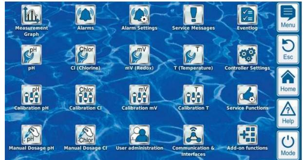
Every function is represented by an icon with supplemental text (The set of icons shown depend on the controller model).
