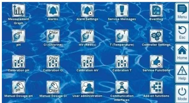
Display and operation are realised on a large TFT colour display with touchscreen. The function shown can be executed with the simple tap of a finger on the corresponding area on the screen. Each tap on the touchscreen is confirmed with a signal tone.
