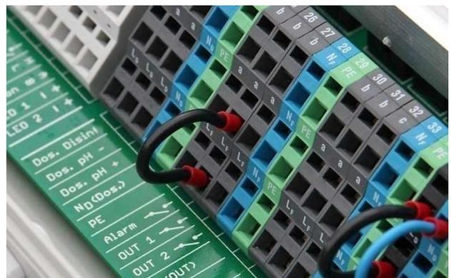
Wire bridge in the terminal box from phase L<sub>F</sub> to centre relay contact a
