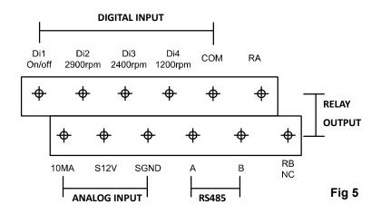
E.g.: To enable external speed control via digital input, connect one of the digits from Di2/3/4 to COM.
