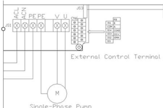
Connectiong of frequency inverter for single-phase Motor 1100/2200
