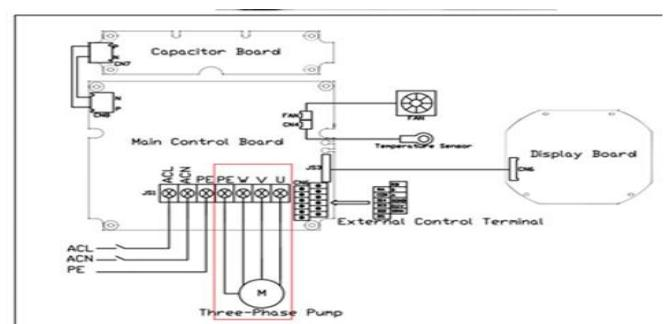
Connection of frequency inverter for three phase Moto (1100C/2200)
